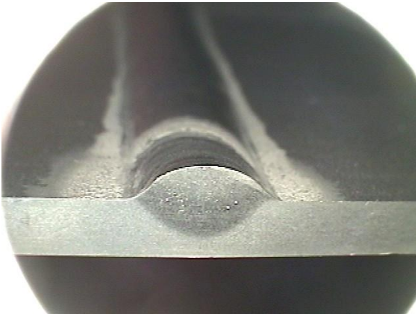
ac-TIG welding (with filler metal)
